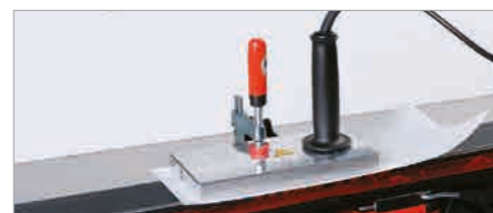
Einkleben mittels Heizplatte und Trennpapier / Glu-in by means of heating plate and anti-adhesive paper / Collez en vous servant de la plaque chauffante et du papier de séparation / Incollaggio tramite piastra termo-elettrica e carta anti-adesiva
